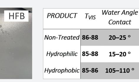
As can be seen in the table above, there is no modification in the transmittance of visible light (TVIS), and the water angle contact is a clear clue of the good performance of each formulation.
