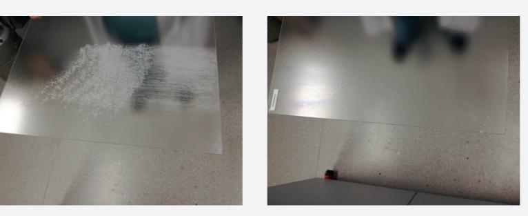
We can observe in the pictures above (non-treated glass on the left and glass with HFL coating on the right) how in the treated sample the talcum powder is completely removed.
