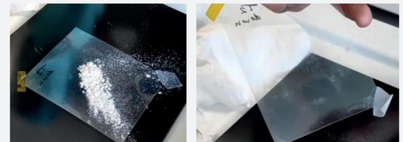
On the one hand, in relation with the reduction of superficial reflections (approach 1), we can see in the picture on the right side how, in the upper part of the glass, the reflection of the light is lower than in the non-treated part.
