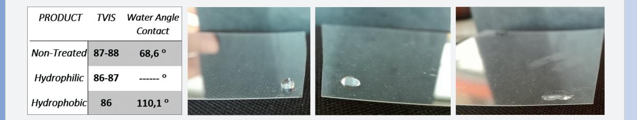
In the pictures above we can observe the situation before and after of the anti-powder effect on flexible sample treated with HFL approach. With this measurement we can observe according to the table how the approach 1 doesn't reduce the transmittance of visible light (only the reflection of incident light) and how the approach 2 increases it.
