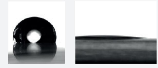
In the pictures on the left it is possible to observe the different water contact angle according to each formulation. The HFB one shows a very clear drop of water meanwhile the HFL approach forms a water film on the glass.
